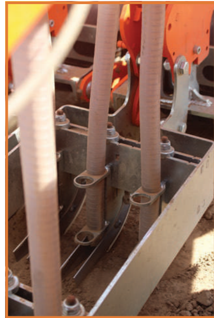
Single pipe delivery into the soil to prevent changes of diameter and potential seed blockage. Space for a second feed into coulter for increased rate or additional product.
