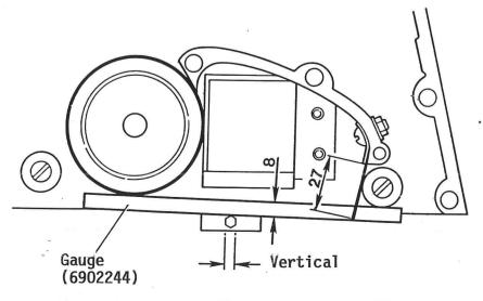
Type B: The pin should be screwed tightly into the attachment plate, with the flats of the hexagon vertical.
